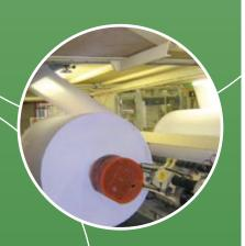
In both slitting and cross cutting operations, the precondition for good winding quality and high format accuracy is a clean cut. All this is dependent on a smooth, crease-free feed of paper webs and even pressure from the pressure rolls to ensure that air is squeezed out. A significant contribution to this are LÜRAFLEX® spreader rolls and LÜRAFLEX® pressure rolls.
