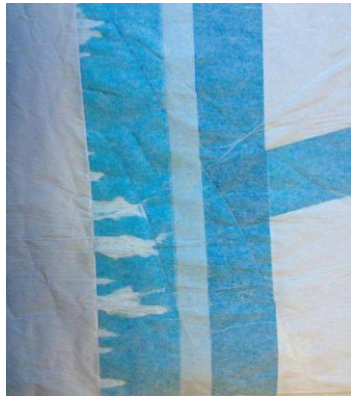
Fig. 8: Adhesive tape with Ink bleeding
