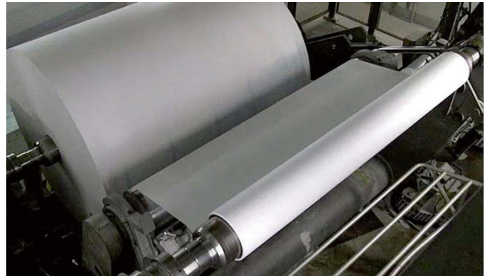
Fig.1: Unwinding of SMS3, Mitsubishi HiTec Paper Europe GmbH, Mill Bielefeld
